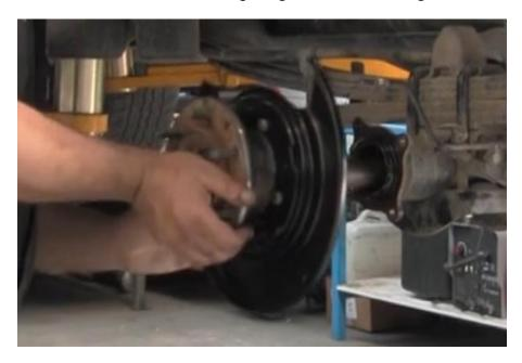
If any oil has leaked from the axle while disassembled, top up the diff oil now.
