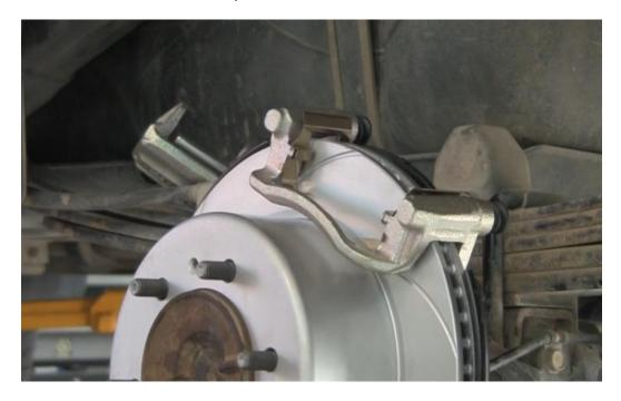
Using the shims supplied #10 make sure the bracket housing is central to the Rotor.
