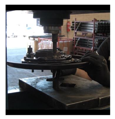
Fit the supplied axle seal to the bearing housing.
